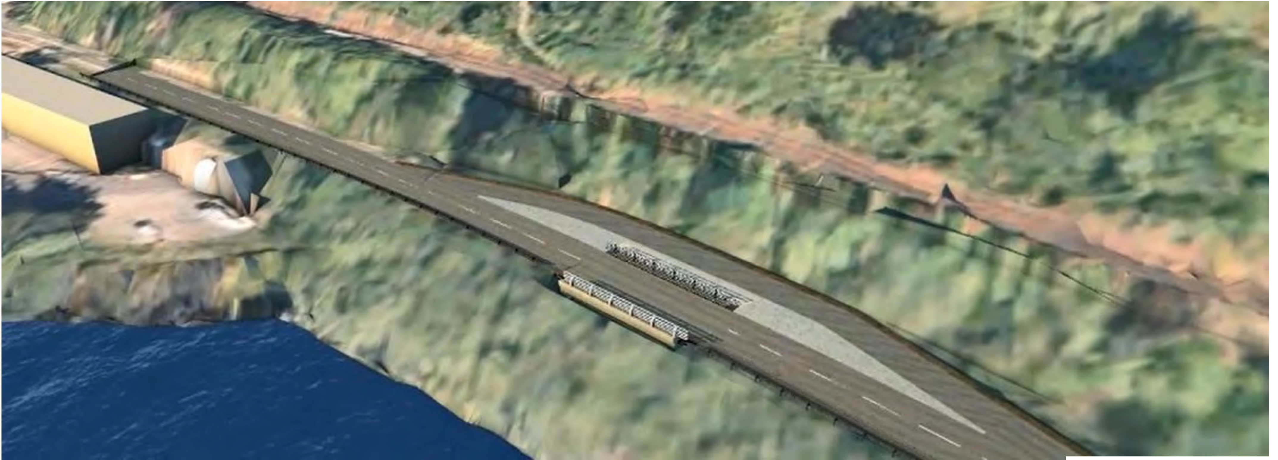
Proposed diversion of A85 into existing layby to facilitate construction of Main Access Tunnel
