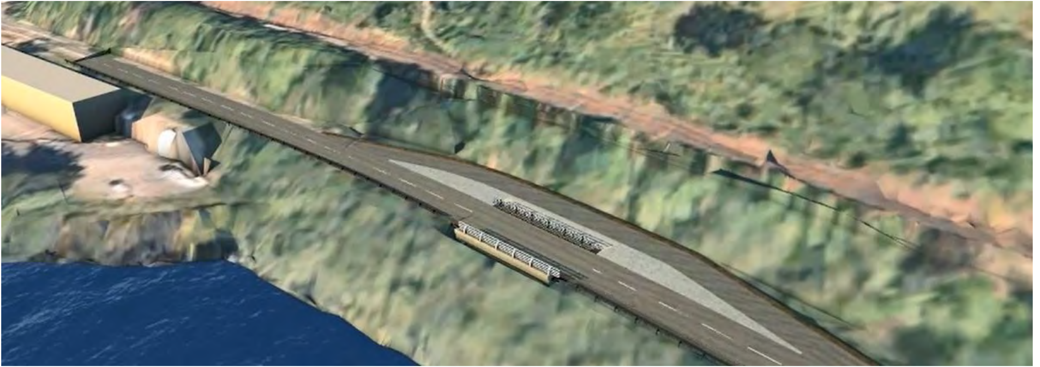
Proposed diversion of A85 into existing layby to facilitate construction of Main Access Tunnel
